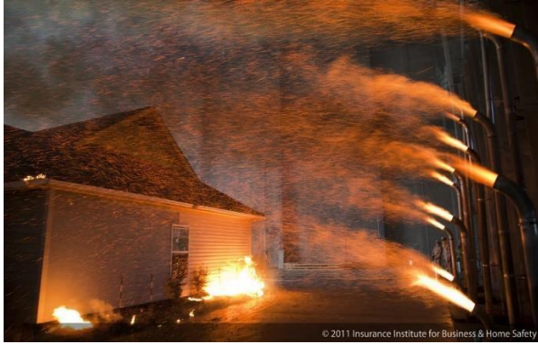
Figure 2: Ember exposure (left) and wind driven rain (right) tests.
