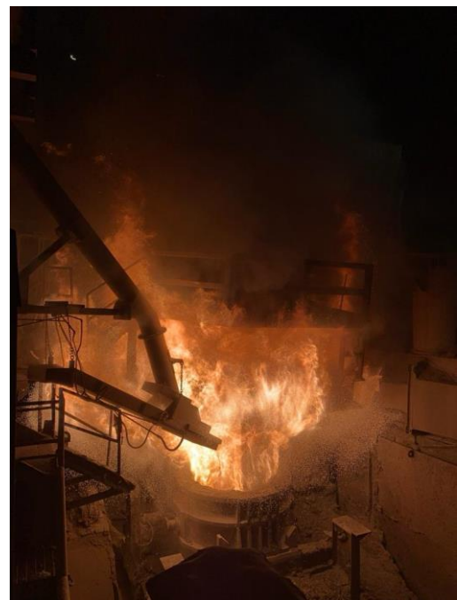
Furnace tapping into ladle with alloys being added through the chute.
