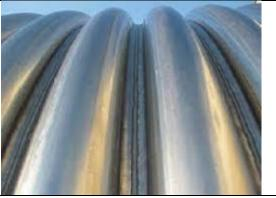
A heat exchange media is passed through the half-pipe and heat exchange is accomplished from the heat exchange media, through the vessel/tank wall, into (or from) the process material. The diagram below illustrates this concept and shows an application where either steam or cooling water is used as the heat exchange media:
