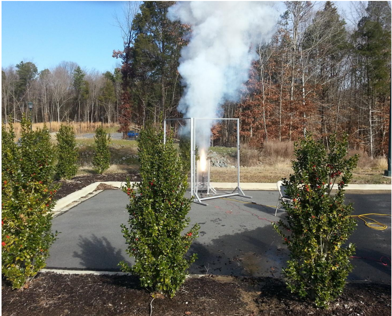
Figure 1: UNCC Solid Fuel Rocket Motor Test Stand
