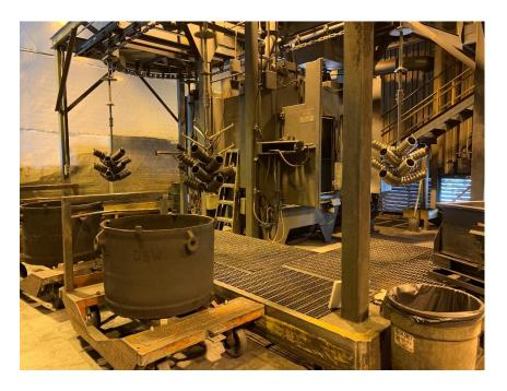
The shot blasting chamber is the back of the photo. Parts (the black ones on the left) are loaded onto steel racks that cycle into the shot blasting chamber. When the cycle is complete, the machine cycles and the freshly blasted parts (silver colored) emerge from the right side and a new batch enters on the left.
