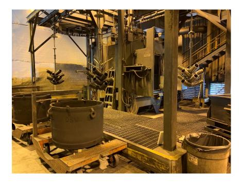
The shot blasting chamber is the back of the photo. Parts (the black ones on the left) are loaded onto steel racks that cycle into the shot blasting chamber. When the cycle is complete, the machine cycles and the freshly blasted parts (silver colored) emerge from the right side and a new batch enters on the left.
