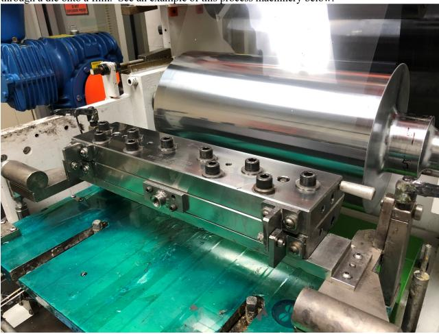
The port in the back of the die receives the coating material. Inside of the die, the material is dispersed through the length of the die, to the front "lip" where it is applied to a rotating roll of substrate film. The following picture shows the inside of the die:
