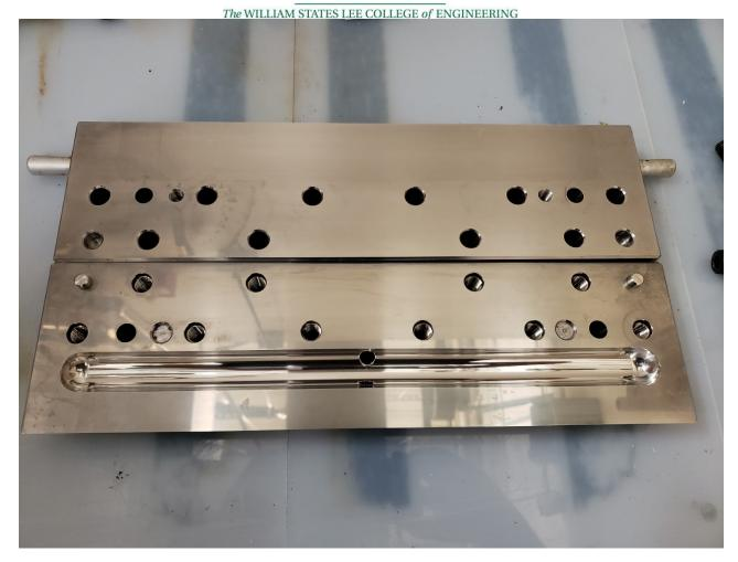
These dies are extremely precise which allows the coating material to be applied to very exacting tolerances.
