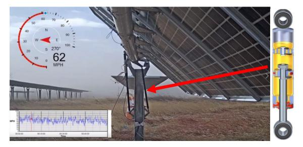
The objective of this project will be design and build a field portable measurement system for determining the amount of oil in a sealed damper.
