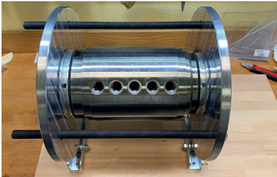
Figure 5: 3 Slot Seal Test Fixture
