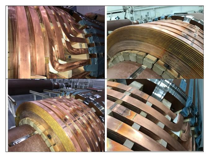
These windings are held secure during the operation with a large metal ring before the rotor enters service:
