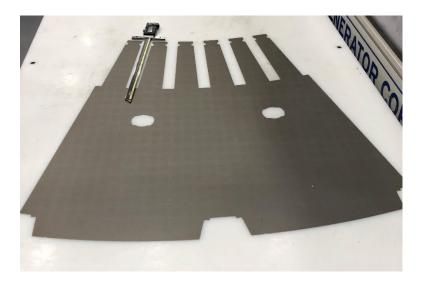
During the manufacturing of a stator core, these laminations are individually stacked to form stator packs (subassemblies of stacked laminations).
