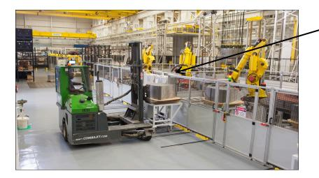
Robotic core stacking of individual laminations or core punchings (stack of laminations on pallet being delivered to robot cell)
