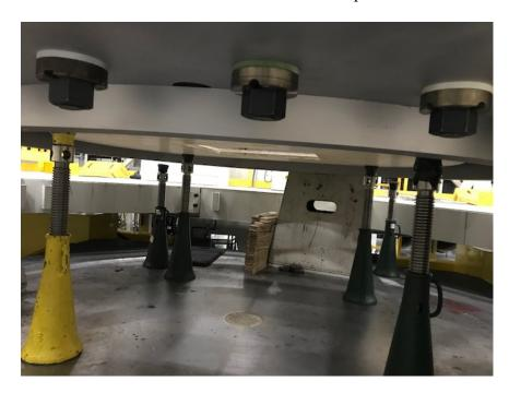
The measurement device is moved through the three positions in the lamination and measurements made with reference to the bottom of the core.
