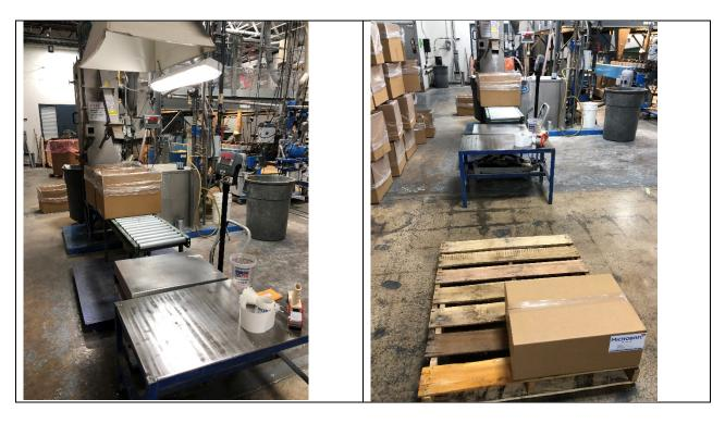
During the process, an operator is required to be present as the boxes are filled and manually moves each box down the line when it reaches the target weight. When the filled box is moved, an empty box is moved into place to start filling and the full box is re-weighed to verify proper contents, then sealed and placed on a shipping pallet.
