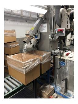
Here is a close up view of the compounded material going into the shipping box:
