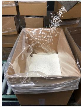
Each box contains a precise amount of compound. This is measured using the weight of the box. An operator monitors the scale and moves the box out of the pellet stream once the scale indicates the weight has been achieved. The next box on the conveyer is then moved by the operator to the filling location. The filled box moves down the line to be sealed and loaded onto a pallet:
