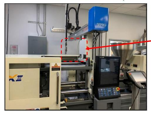
Mold lifted into this area and then lowered into place
