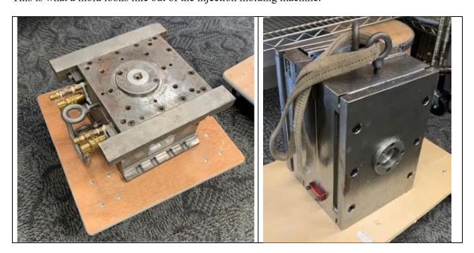
These molds can weigh up to 500 lbs. They all have lifting eyes as shown in the photos. The
