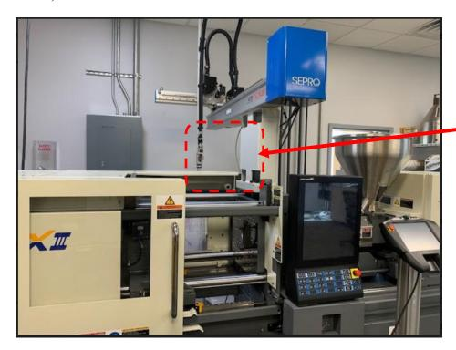
Mold lifted into this area and then lowered into place
