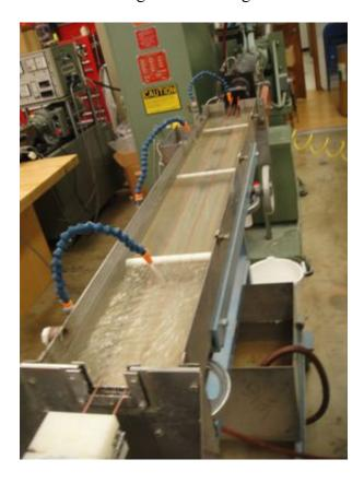
The water temperature, the speed of the line through the water and the length of the tray are all elements to be designed based on the size and chemical composition. Some materials are hydrophilic and the absorption of too much water can ruin their composition.
