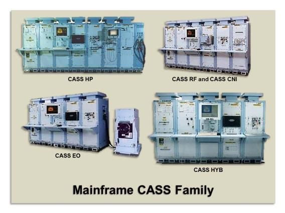
While at sea or ashore, maintainers are able to connect avionics systems to an eCASS station, run a set of automated tests that identifies the problem, and perform the necessary maintenance to fix the issue. Once the maintenance is complete, the avionics are reconnected to the eCASS station to verify that the problem is fixed and the avionics are ready for flight.
