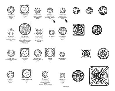
Occasionally, a harness will develop a short or continuity issue. If a harness is suspected of being faulty, mechanics remove the harness from the aircraft and use a multi-meter to complete pin-to-
