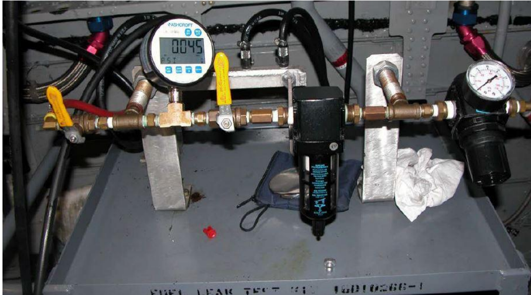
Current Pressure Test Set used to test the H-53 Fuel System.
