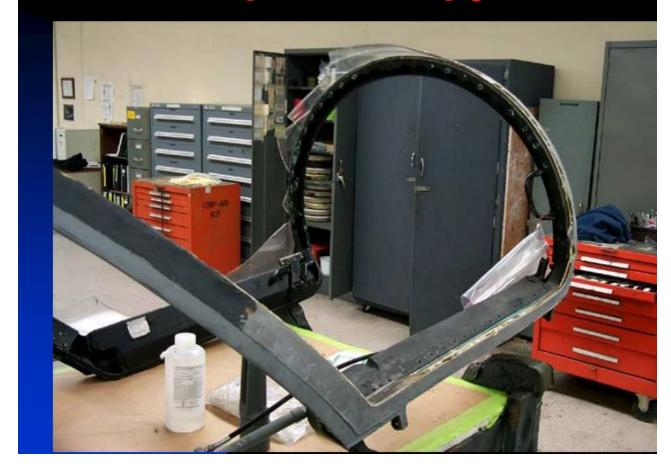
The inspection occurs every 50 flight hours using a prism, flashlight and glycerol. The prism and glycerol are used to look into the transparency edge block to find horizontal/vertical cracks.
