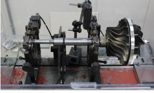
This machine spins the rotor shaft and measures the balance of the unit. When complete, it provides and output which indicates if the unit is in balance or not:
