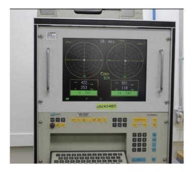
If the unit is not in balance, the output provides a location and amount of material that must be ground away to rebalance the shaft.
