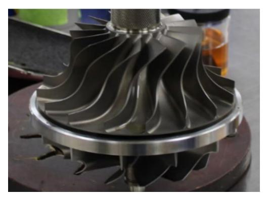
The Compressor Wheel is attached to the rotor shaft. Due to the high speed operation, it is critical that the assembly is balanced. Checking this balance is one of the critical maintenance operations when the APU's come in for service.
