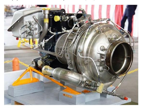
APU's are gas turbine engines used on aircraft to provide power when the aircraft is on the ground to do such things as operating hydraulic and electrical systems to check their operation. This
