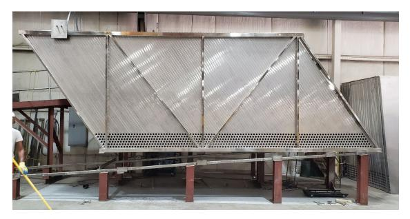
When plates are ready to be assembled into the plate pack system, two operators lift the plate off of the storage rack and carry it to the nearby plate pack frame and manually insert it into the frame and move it into the proper depth and angle orientation. Over the course of a shift, the operators may move up to 300 plates.
