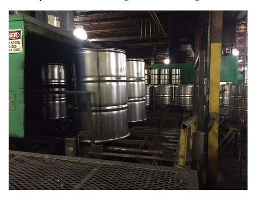
In this photo, the two drums that just exited, have proceeded down the single lane conveyer rollers and two new drums are exiting the washer.
