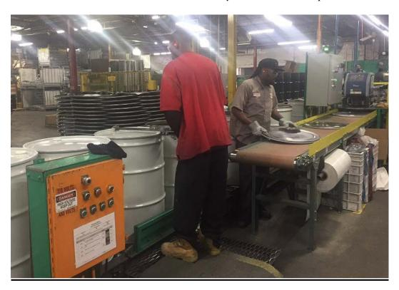
When the drum enters the operation, the station equipment grabs the drum and keeps it stable during the cover removal. The tool shown in the picture is used to loosen the cover and then the cover is lifted off the drum:
