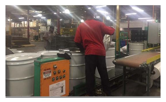
The project intent is to produce a working automated machine that removes the cover from the drum and places the cover upside down on a belt conveyor. The current process is manual and needs to move to an automated station. The cover is crimped on. This requires the cover to be popped off, picked up, flipped, and placed on the next process belt. The unit must operate with a throughput of no less than 10 per minute and be fully automated.
