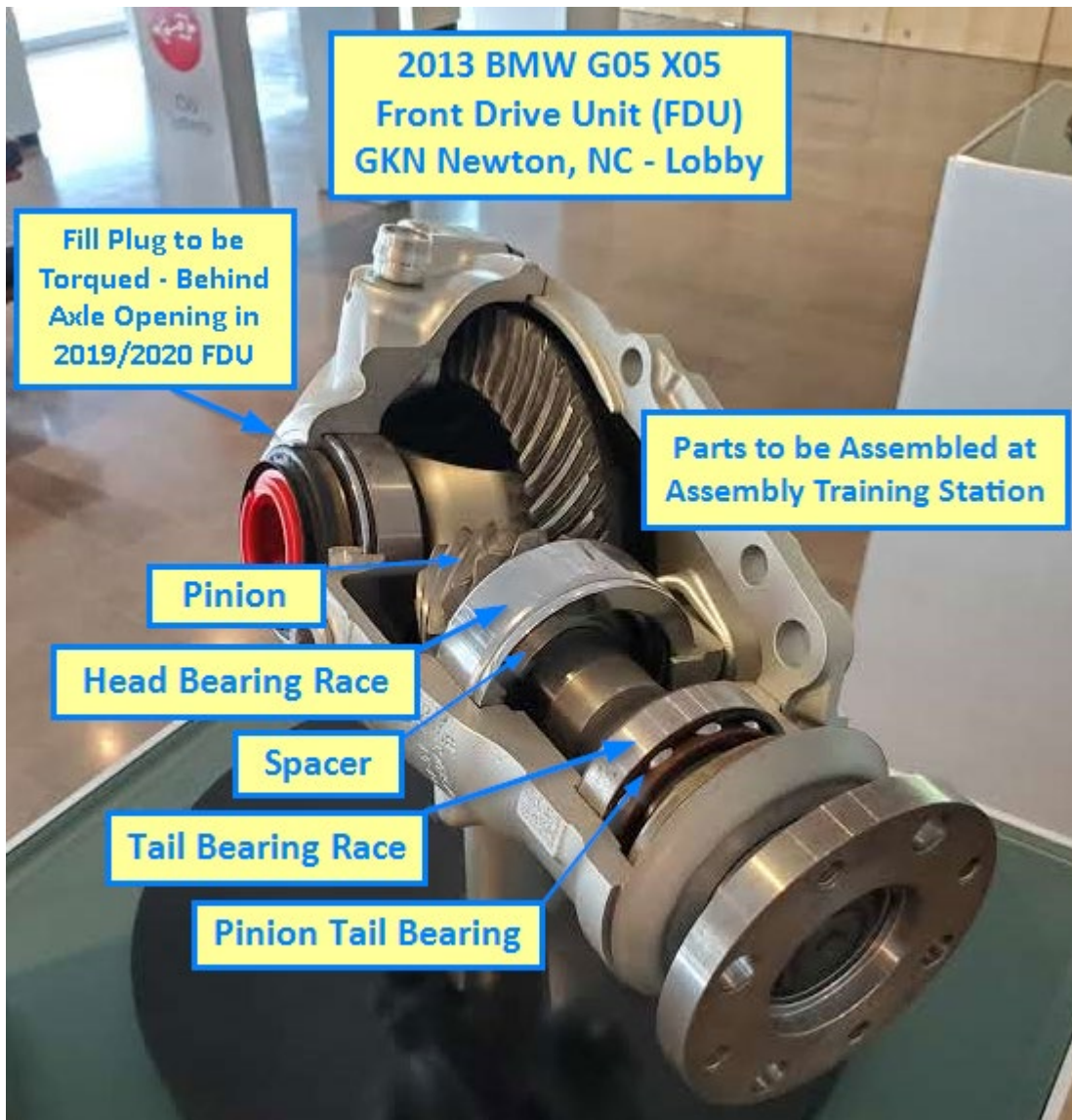
Figure 1 – Parts from the BMW G05 X05 Front Drive Unit to be Assembled at the Training Station
