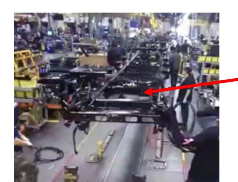
Frame assembly being carried by hoist to moving line
