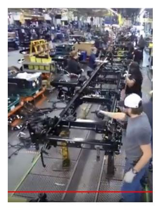
In the photo above, the frame is in the pedestal conveyor and the assemblers start conveyer line assembly.
