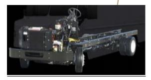
The units has an engine, drive train, frame, axles, wheels and a steering wheel. It does not have a body with a seat. The unit is drivable and driving it to the next location in the process is the most convenient way to move the units. Since there is no seat the operators clamp a temporary seat onto the frame rail so they can drive the unit to the next station in the process. See temporary seat in the photo below:
