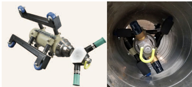
Figure 2: Abrasive Blasting Skid – Pipe Cleaning
