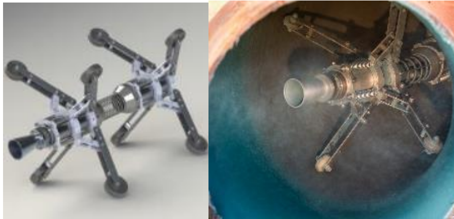
Figure 1: Spin Cast Skid – Liner Application
