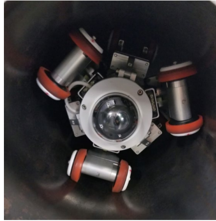
Figure 3: In-Pipe Visual Inspection
