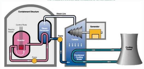
A key piece of equipment in this system is a steam generator which contains long bundles of densely packed (gap between tubes is <0.2") tubes that range in diameter from 0.625 to 0.875". Tube bundles can contain between (3500 to 10,000) individual tubes. The figure below shows a more detailed view of the steam generator:
