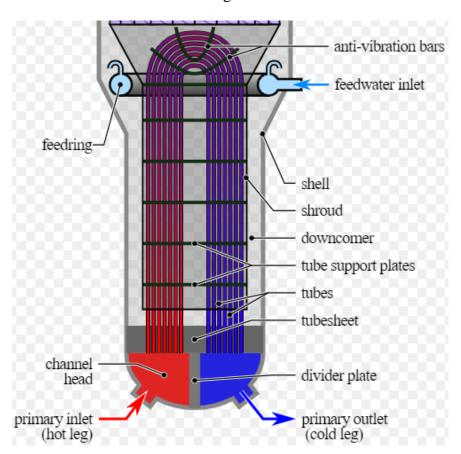
Foreign material can get into the tube bundle areas and damage the tubes. Periodic inspections are made to look for foreign material and damage that may be caused by foreign material when
