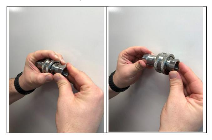
In this example, the locking collar is retracted, which allows full insertion of the part on the right side. Once seated, the collar is released which locks and seals the coupling in place.
