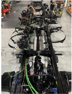
Chassis with air lines and electrical harness installed (6 stations after previous picture)
