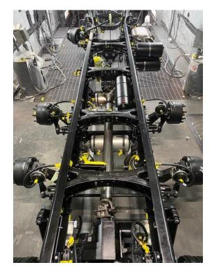
Chassis without air line bundle and electrical harness (prior to entering chassis paint process)
