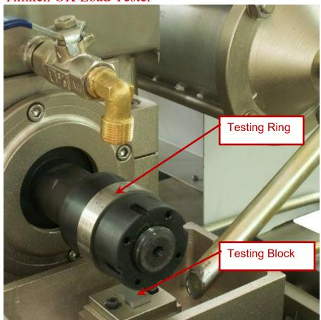
Experience has shown that standardized wear tests like block-on-ring provide a reasonable indication of adhesive wear performance but do not adequately simulate the complex forces seen in real pump service. Coatings that held promise in small-scale testing would inexplicably fail or delaminate during pump testing. Without a more economical method to screen for these complex failures it is difficult to take advantage of many of the new surface treatment technologies available in the marketplace.
