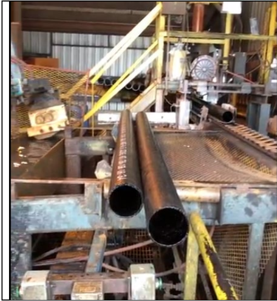
Pipe entering the test station
