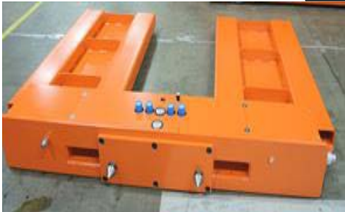
Air “Bladders” mounted under the pallets
