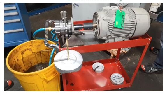
The work for this project will be to take that test rig and design and implement changes so that it can be fully utilized for the purpose of wear testing.
