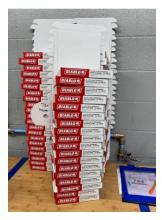
**Current status:** blade insert is added to the carton then manually count 10 pcs and manually place a sheet protector / between each blade. Manually verify count by weigh counting with scale, visually check the presence of the UPC and warning label.
