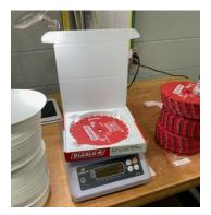
**Current state:** manually close the carton, pick tape from the auto dispenser, tape close and slide the carton over to the master pack table.
