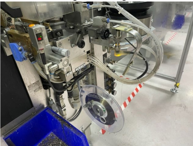
Solder Reel feeding into brazing machine:
