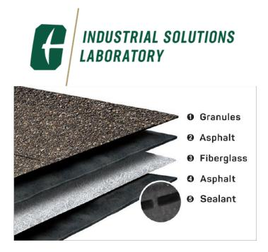
These materials are produced in large factories with continuous roll lines including applications of "whitewater" in the nonwoven mat production, molten liquid asphalt, and bitumen granules. Amazingly, these products can be warrantied for 25 years or more!
